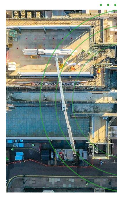
This crane will lift a maximum load of 12 tonnes with a 5m radius and an impressive maximum radius of 45 meters with 100 kg or 34 m with 1,000 kg load. The Böcker 52 is equally impressive with an extremely large working area.
