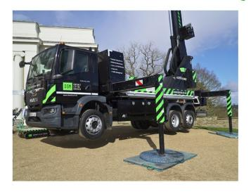
With a 52-metre maximum extension and a 6,000kg lifting capacity, the AK48 excels in both high-reach and precision lifting scenarios. Its lightweight aluminum boom ensures exceptional reach while maintaining optimal manoeuvrability. The hybrid drive system seamlessly switches between electric and diesel power, reducing emissions and lowering operational costs.
